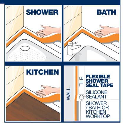
Position the bath, tray etc against the wall and bond the top part of the tape to the wall with a suitable product (Larsen F1X, Larsen Tanking membrane or suitable Larsen cement based tile adhesive).
